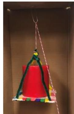
In designing their cranking device to serve as a motor, students can use a dowel rod or stiff straw to serve as the shaft that spins to wind up or wind down the cable. If they attach a popsicle stick or similar structure to one end, this makes the lifting easier as they gain a considerable mechanical advantage (if your students are at the appropriate level you can also calculate the mechanical advantage). It also helps to use tape to secure the cranking device to the floor or table.
